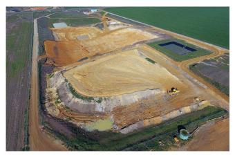
The landfill site showing the current cell approaching capacity in the foreground, with the new cell under construction in the background
