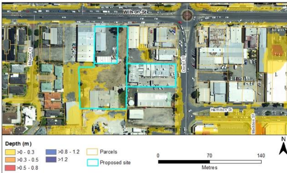
Figure 2: The proposed site highlighted on a property cadastre layer showing the extent of stormwater inundation and depths resulting from a 1% AEP flood event.
