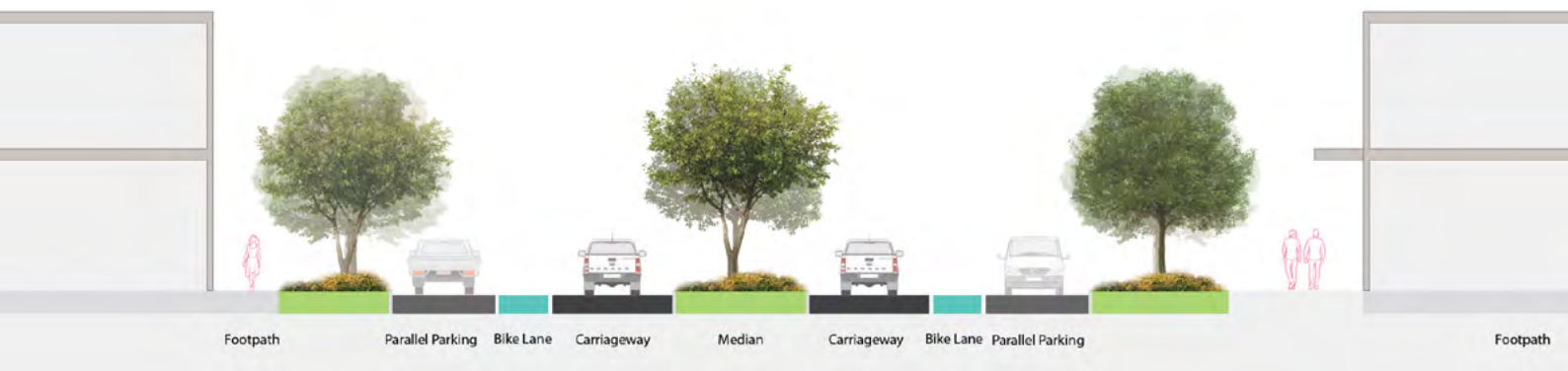
Figure 23 - Proposed upgrades in Darlot Street - Typical Section
