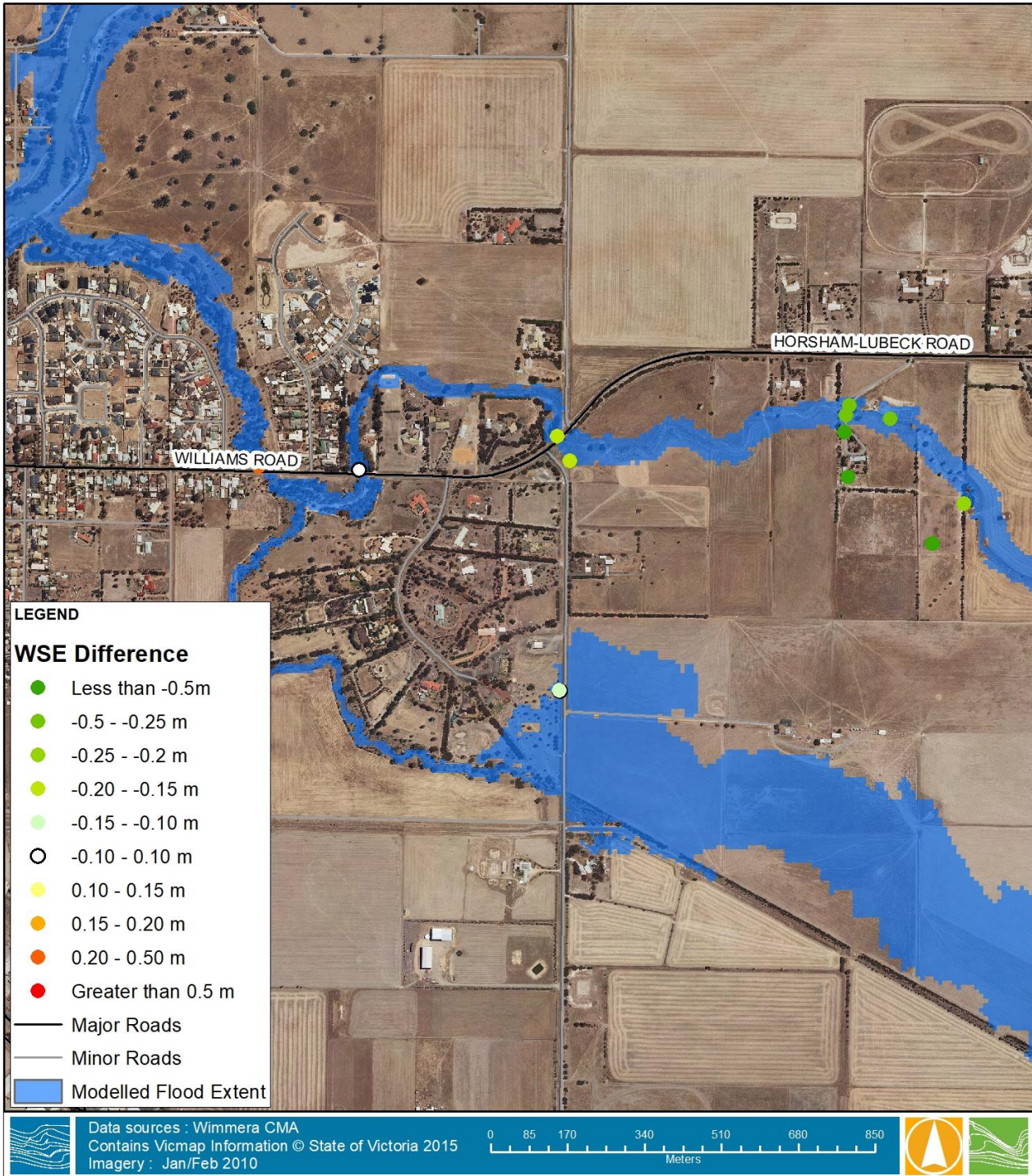
FIGURE 4-39 SEPTEMBER 2016 MODELLED AND SURVEYED LEVEL COMPARISON – LOWER BURNT CREEK
