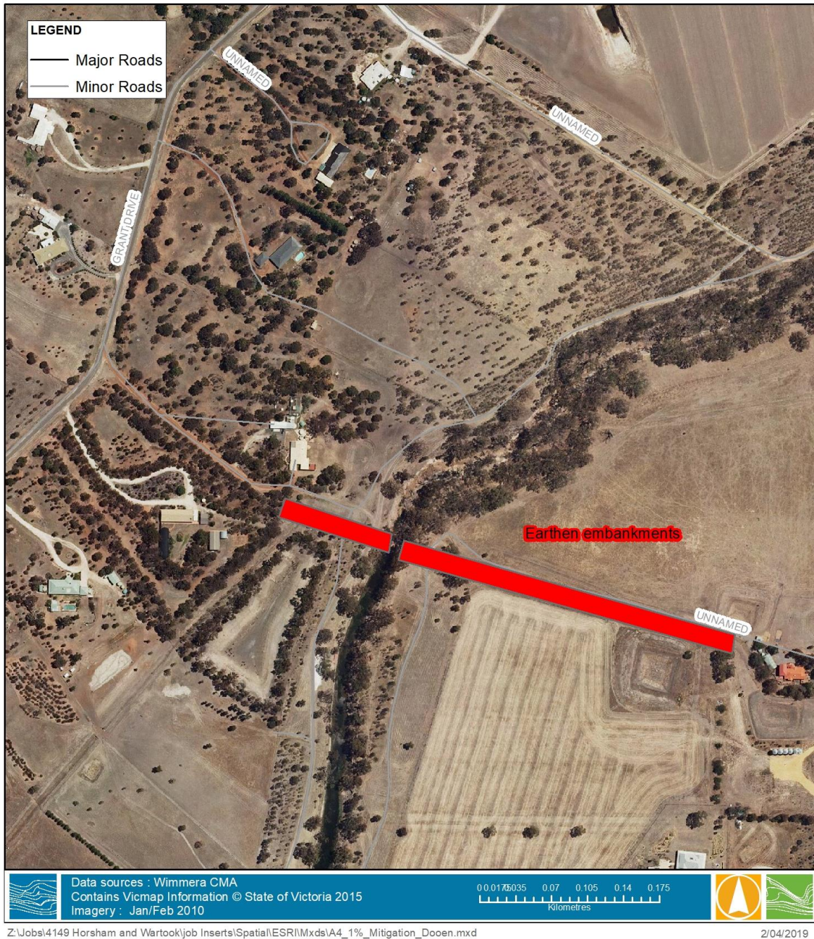
FIGURE 5-26 DOOEN SWAMP CAPACITY RESTRICTION EMBANKMENTS
