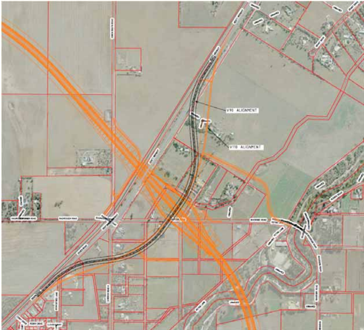
Figure 3 Proposed modified alignment for the Henty Highway interchange ( AECOM Plans SKE-0004 & SKE-0005 )
