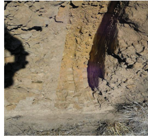
Lot 7 Soil Test Category 5 Clay Soil at 75mm
