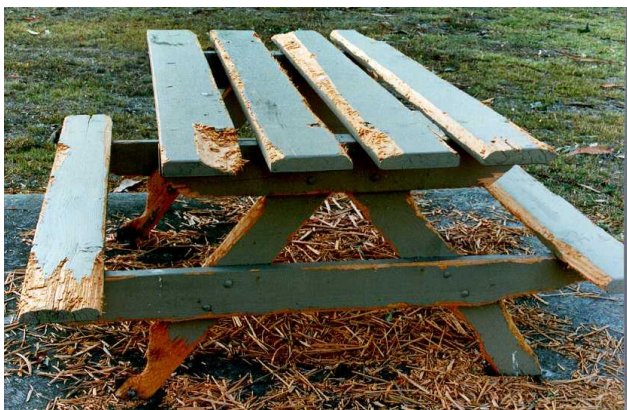
Figure 6: Cockatoo damage to outdoor furniture
