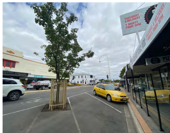
Trees on Firebrace Street are under-performing due to soil and root compaction and poor drainage.
