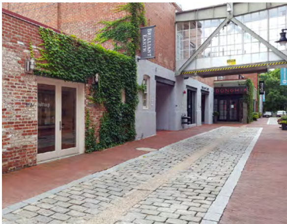
A shared street with flush kerbs demarcating space
