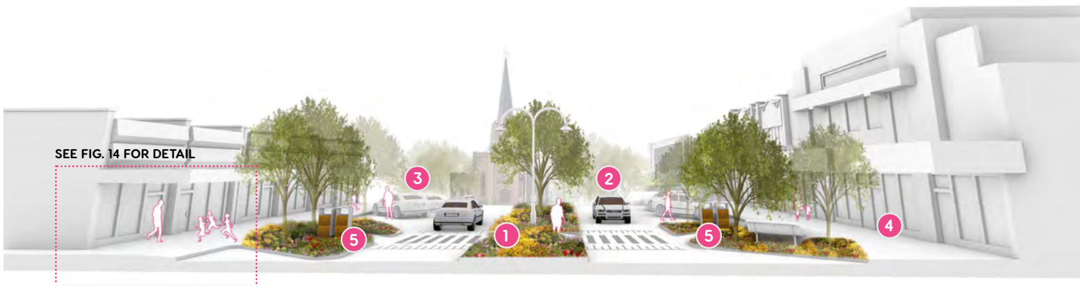
Figure 13 - A widened planted median in Firebrace Street will provide consistent canopy without impacting on existing angled parking
