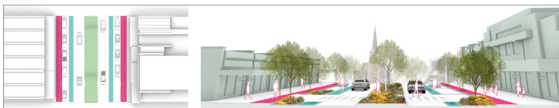
Scenario C Plan - A widened median and bike lane along Firebrace Street
