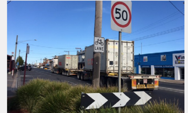
Wilson St (looking east) – Bicycles coexist with heavy vehicles in a lane that lacks both separation and protection, positioned behind angle-parked cars.
