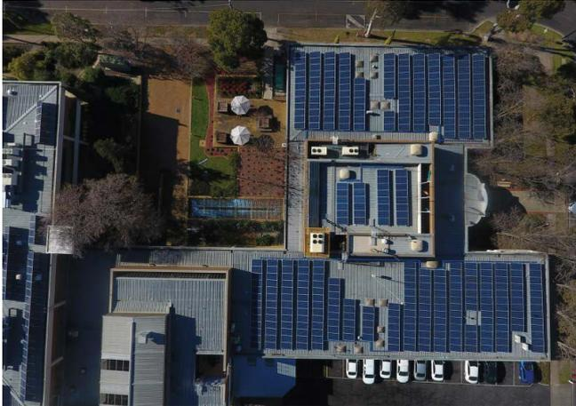
As a way of reducing energy consumption, 99kw of solar panels were installed on the roof of the Civic Centre Municipal Office this year
