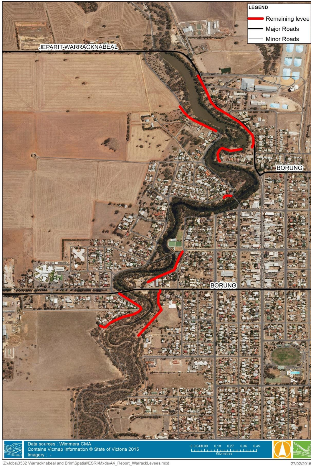
Figure 1-11 Warracknabeal Remnant Levees
