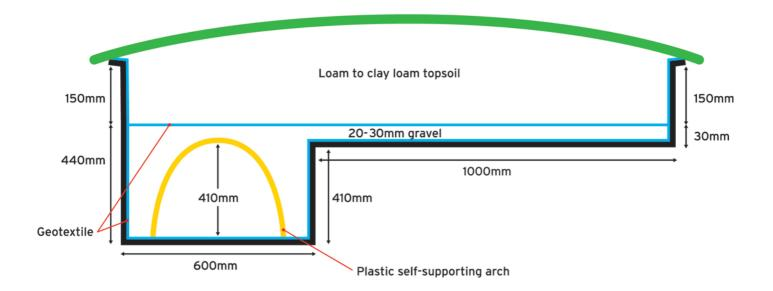
For secondary treated effluent
