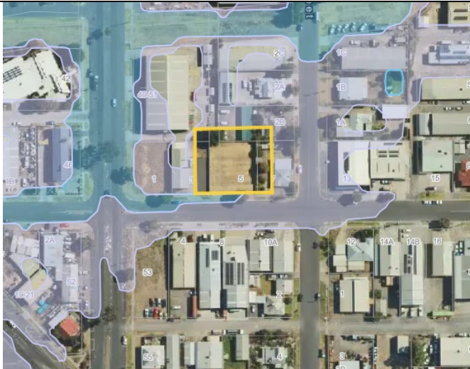
Figure 2 Map 13LSIO-FO– Current (incorrect) mapping of Floodway Overlay and Land Subject to Inundation Overlay as it appears in the Horsham Planning Scheme (Flood Overlay – blue, Land Subject to Inundation Overlay – light blue, area highlighted – mapping error)
